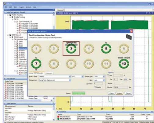
Infinity's Acquisition Wizard uses ASSIST Technology to automatically detect connected sensors and verify their operability.
